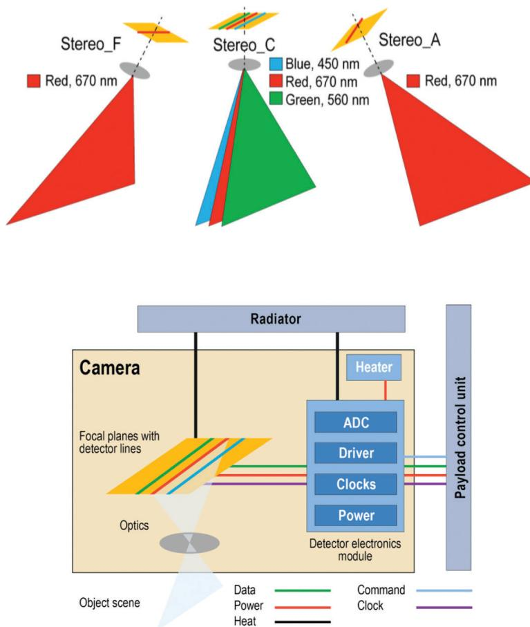
**Fig. S2. MAI. (top) Instrument concept. (bottom) Top-level architecture for its cameras. ADC is analog-to-digital converter.**
