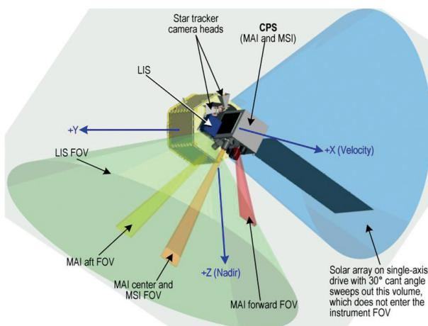
**FIG. S1.** The CHASER spacecraft uses high-heritage components, resulting in a low-risk mission.
