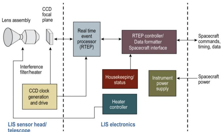
**FIG. S4. LIS Functional block diagram. CCD is charge-coupled device.**
