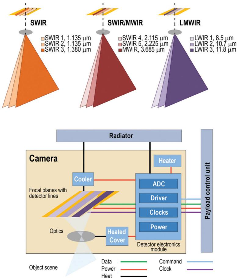
**FIG. S3. MSI. (top) Instrument concept. (bottom) Top-level architecture for its cameras.**
