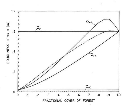
Figure 1: Roughness lengths as a function of fractional cover of forest.  $Z_{0eff}$ : effective roughness length reflecting form drag and total skin drag,  $z_{0e}$ : effective roughness length due to total skin drag,  $z_{01}$ ,  $z_{00}$  roughness length of forest and open field. Dashed line: effective roughness length  $Z_{0eff}$  reflecting form drag and total skin drag, but computed with a blending height of  $l_b = 5m$  in Equations 3, 5, 6.
