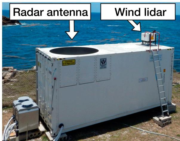
FIG. 1. The 35.5-GHz (Ka band) polarized Doppler cloud radar, located at the BCO. The container walls act as a clutter fence for the 2-m-diameter antenna dish. A wind lidar is mounted on the right side of the roof.
