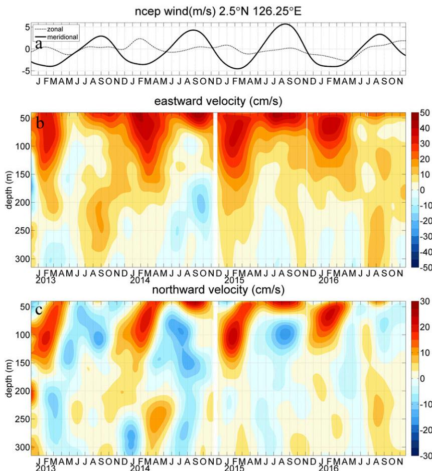
FIG. 2. NCEP (a) winds ( $\text{m s}^{-1}$ ) and the (b) zonal and (c) meridional components of the moored ADCP velocity ( $\text{cm s}^{-1}$ ) time series at M00 in the Maluku Channel during December 2012–November 2016.
