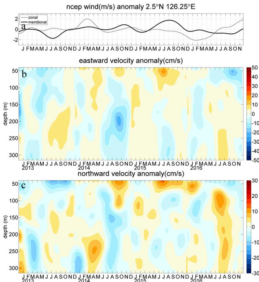
FIG. 4. NCEP (a) winds anomalies ( $\text{m s}^{-1}$ ) and (b) zonal and (c) meridional current anomalies ( $\text{cm s}^{-1}$ ) at station M00 in the Maluku Channel relative to the climatology of 2013–16.
