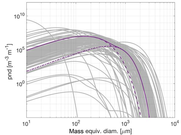
**Figure 1.** Size distributions for the idealized mean profile (purple) and 90 simulated profiles (grey) derived from ICON at 550 hPa each. The sum of the distributions for IWC and SWC is shown for all profiles, and the individual distributions for IWC (dashed) and SWC (dash-dotted) are shown for the mean profile.
