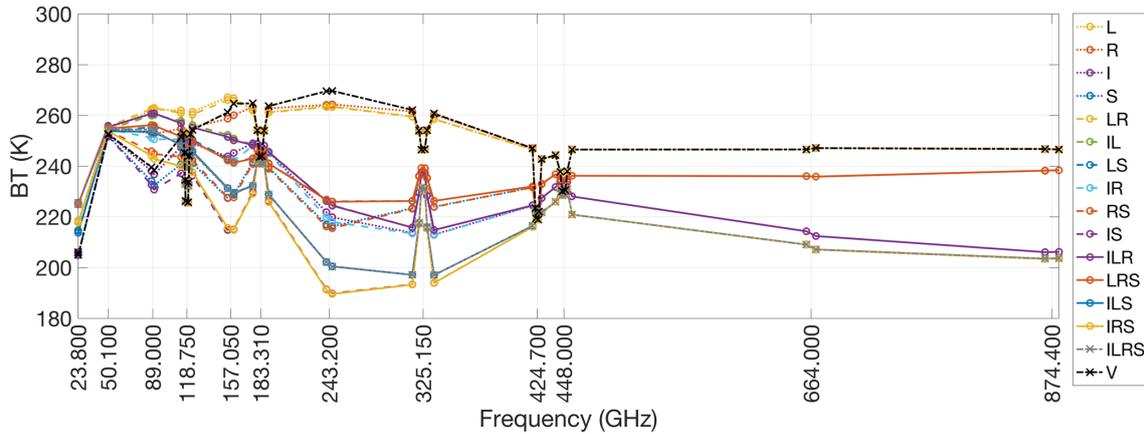
**Figure 4.** Brightness temperature spectrum for  $\epsilon = 0.6$  for the 16 combinations of the base profile. The legend corresponds to the composition suffixes X defined in Table 3. The labels on the abscissa are the centre frequencies of the channels. The curve labelled “V” is for H<sub>2</sub>O only, without any hydrometeors. Although not mentioned in the legend, vapour is also present in all the other calculations.
