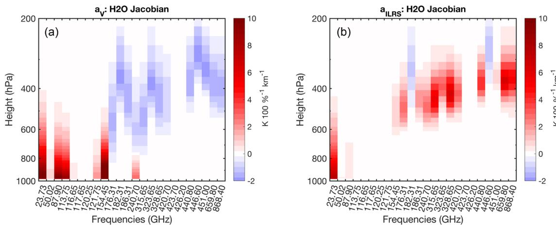
**Figure 5.** H<sub>2</sub>O Jacobians for the clear sky case  $a_v$  (a) and for the all-hydrometeor case  $a_{ILRS}$  (b) for an emissivity  $\epsilon = 0.6$ . Averages of the sidebands are shown, the labels on the abscissa denote the left sideband of the channel.
