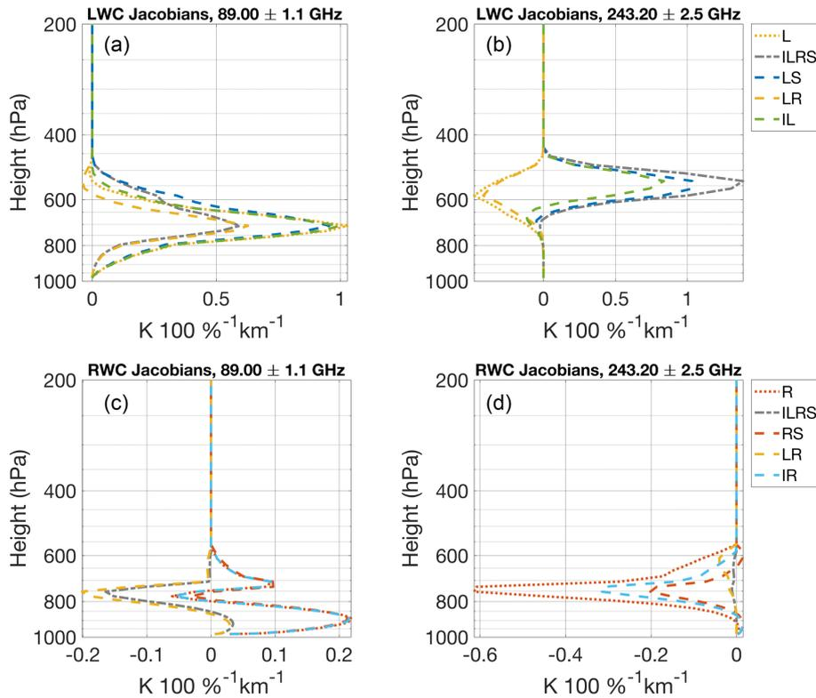
**Figure 8.** LWC (a) and RWC (b) Jacobians for the 89.0 GHz (a, c) and the 243.2 GHz (b, d) channel ( $\epsilon = 0.6$ ). Shown are atmospheres containing pairs of hydrometeors and the all hydrometeor case  $a_{ILRS}$ . The labels in the legend correspond to the atmospheric composition suffix X. Note different values on the abscissa in the different plots.
