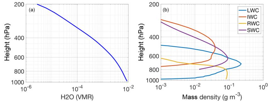
**Figure 3.** Idealized atmospheric base profile. H<sub>2</sub>O volume mixing ratio (VMR, **a**) and particle mass densities (**b**) for LWC, IWC, RWC and SWC. The respective paths are LWP = 0.45 kg m<sup>-2</sup>, IWP = 0.17 kg m<sup>-2</sup>, RWP = 0.18 kg m<sup>-2</sup>, SWP = 0.30 kg m<sup>-2</sup> and H<sub>2</sub>O path = 25.00 kg m<sup>-2</sup>.
