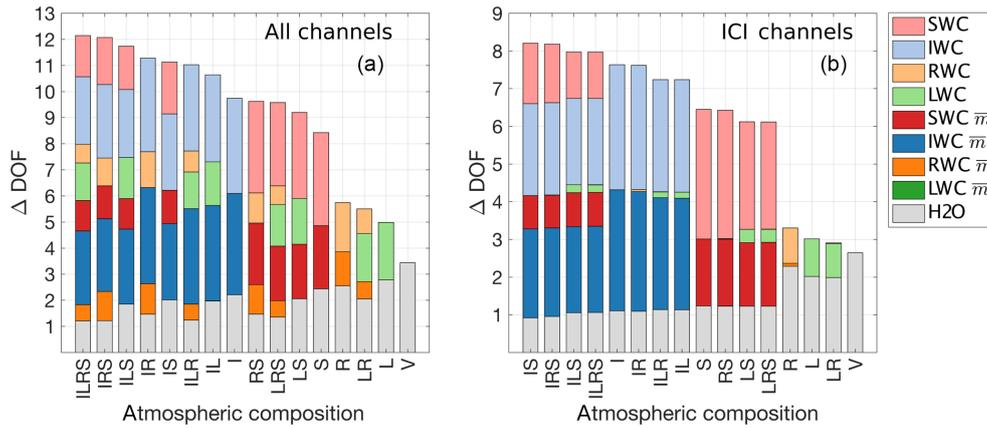
**Figure 10.** Information content  $\Delta$ DOF for all atmospheres, ranked according to the total  $\Delta$ DOF. Results for the full set of channels are shown on the left, results for channels corresponding to ICI are shown on the right. Both were calculated with  $\epsilon = 0.6$ .
