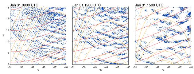
FIG. 3. Cloud lines at the time shown above each panel (gray) and 30 min later (blue). Colored areas mark brightness temperatures between 290 and 293 K in the GOES-E 10.3- $\mu$ m infrared band. Overlaid are streamlines of ERA5 horizontal winds averaged below 500-m altitude (red) and streamlines indicating the shear vector between the surface and 1500 m (yellow).
