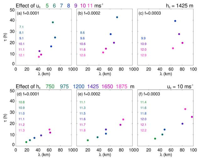
FIG. 5. Numerical solution to Eq. (13). Shown is doubling time vs horizontal wavelength for (left) f = 0.0001, (center) f = 0.0002, and (right) f = 0.0003 for (a)–(c) the effect of changes in  $u_0$  at constant  $h_0 = 1425$  m and (d)–(f) the effect of changes in  $h_0$  at constant  $u_0 = 10$  m s<sup>-1</sup>. Filled circles mark the minimum of  $\tau$ . The corresponding phase velocities are listed in each panel.
