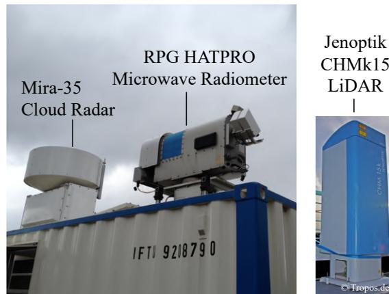
**Figure 2.7.:** LACROS supersite container located at a sewage plant near Krauthausen with all Cloudnet instruments, the lidar was installed at the surface near the container, modified from Hansen (2014).
