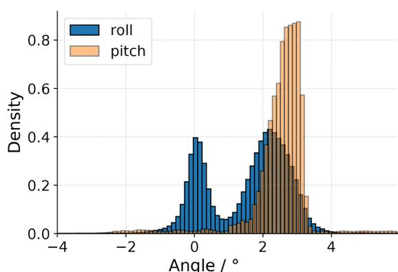
**Figure 5.** Distribution of roll and pitch angles for all HALO flights during EUREC<sup>4</sup>A.
