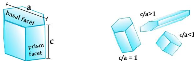
Figure 2.3: Basic shapes of ice crystals. The axial ratio  $c/a$  defines the shape of the crystal: less than 1 for plates-like, greater than 1 for columnar.
