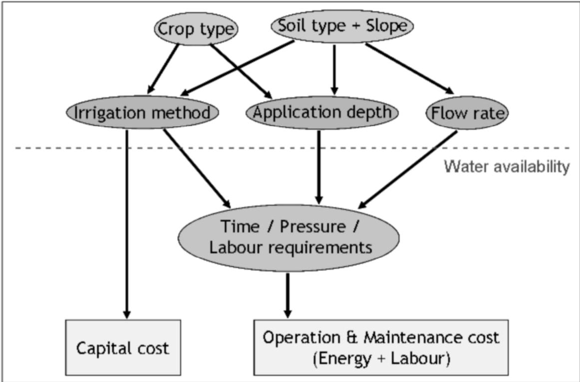
Figure 1: Scheme for determining total irrigation costs
