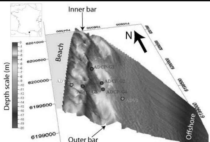
Figure 1. Bathymetric map of the study zone, showing the system of double bar of Leucate Beach and the position of the instruments during the hydrodynamic campaign (ADCPs in red and ADVs in green).
