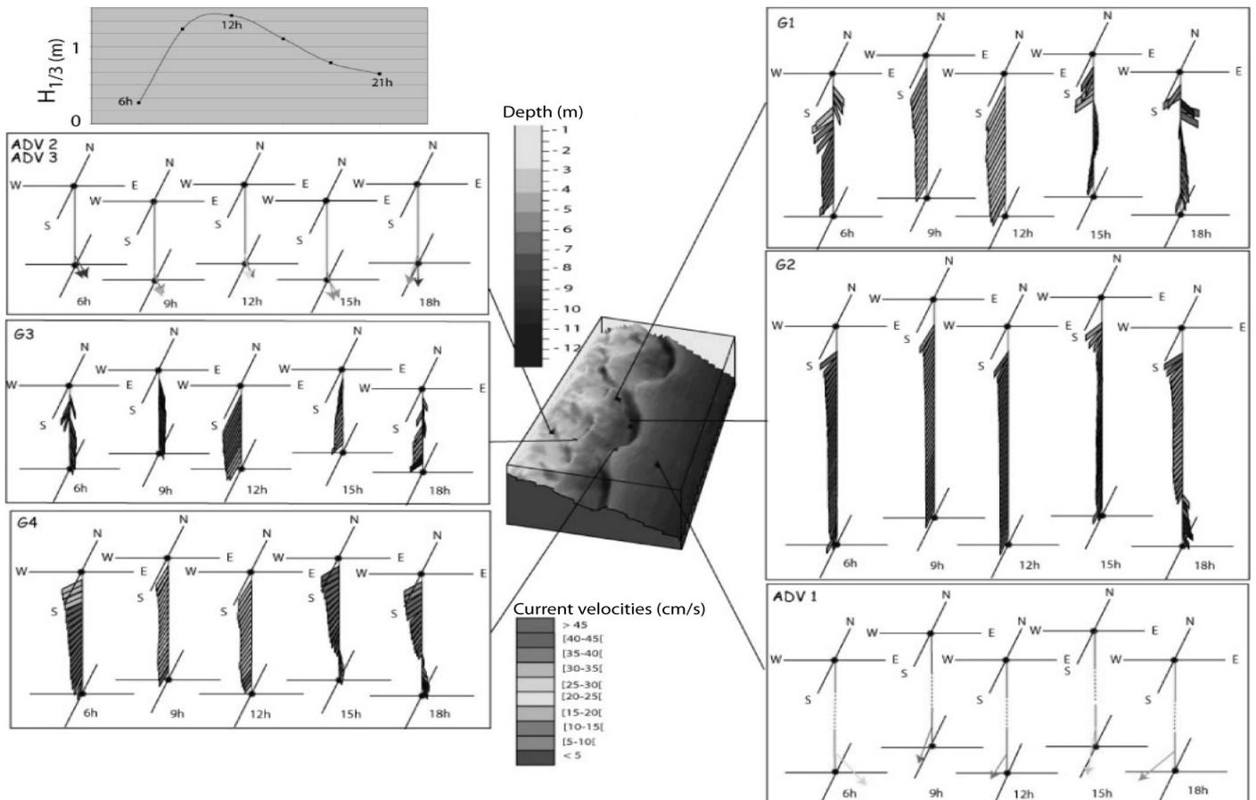
Figure 3. Hydrodynamic map of the currents profiles over Leucate Beach bar system during the 25/01/2007 event, based on ADCPS measurements and ADVs.
