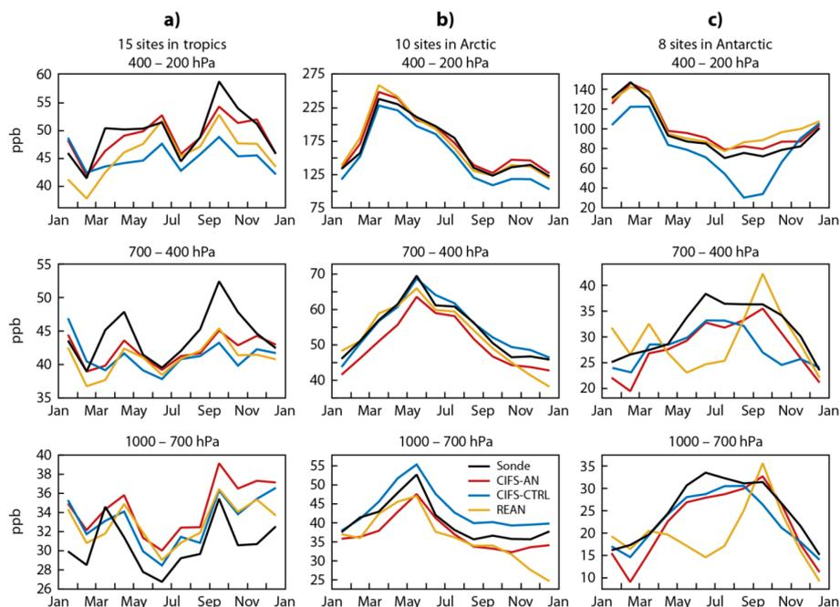
**Figure 15.** Time series of monthly mean tropospheric O<sub>3</sub> in ppb over (a) tropics (15 stations), (b) Arctic (10 stations) and (c) Antarctic (8 stations) averaged in the pressure bands 1000–700 hPa (bottom), 700–400 hPa (middle) and 400–200 hPa (top) from ozonesondes (black), CIFS-AN (red), CIFS-CTRL (blue) and REAN (orange) in 2008.
