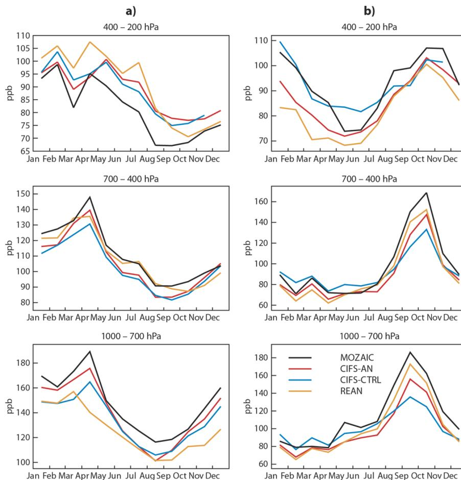
**Figure 5.** Time series of monthly mean tropospheric CO in ppb over (a) Frankfurt (50° N, 8.6° E, 837 profiles) and (b) Windhoek (22.5° S, 17.5° E, 323 profiles) averaged in the pressure bands 1000–700 hPa (bottom), 700–400 hPa (middle) and 400–200 hPa (top) from MOZAIC aircraft data (black), CIFS-AN (red), CIFS-CTRL (blue) and REAN (orange) in 2008.
