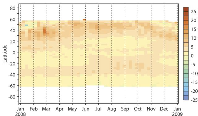
**Figure 19.** Time series of weekly averaged zonal mean OMI TRCNO<sub>2</sub> analysis increment (analysis minus forecast) in % for 2008. Red indicates positive values, blue negative values.
