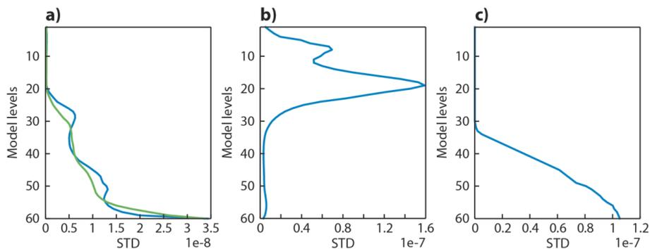
**Figure 1.** Background error SD profiles (blue) at 50° N, 10° E for (a) CO in kg kg<sup>-1</sup>, (b) O<sub>3</sub> in kg kg<sup>-1</sup> and (c) log(NO<sub>2</sub>), dimensionless. Also shown in (a) is the profile for the CO background error SD of the original MACC system used in REAN (green).
