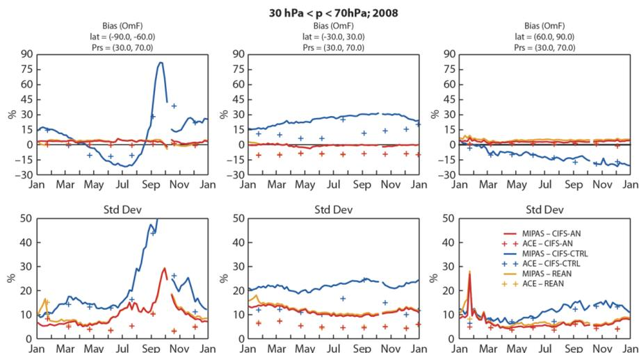
**Figure 13.** Time series for 2008 of monthly mean differences (top) and SD (bottom) in % of the experiments, ACE data (plus symbols) and MIPAS data (solid) averaged over the pressure range between 30 and 70 hPa, for the Antarctic (90 to 60° S, left), the tropics (30° S to 30° N, centre) and the Arctic (60 to 90° N, right). CIFS-AN is shown in red, CIFS-CTRL in blue, and REAN in orange.
