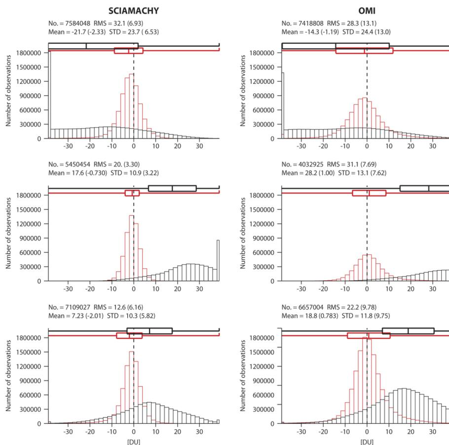
**Figure 8.** Histograms of SCIAMACHY (left) and OMI (right) TCO<sub>3</sub> analysis departures in DU for CIFS-AN (red) and CIFS-CTRL (black) for 2008 averaged over the NH (90–20° N, top), the tropics (20° N–20° S, middle) and the SH (20–90° S, bottom) for all good data. Also shown above the panels are the number of observations that make up the average, as well as the mean, RMS and SD of the departures with values for REAN in brackets.
