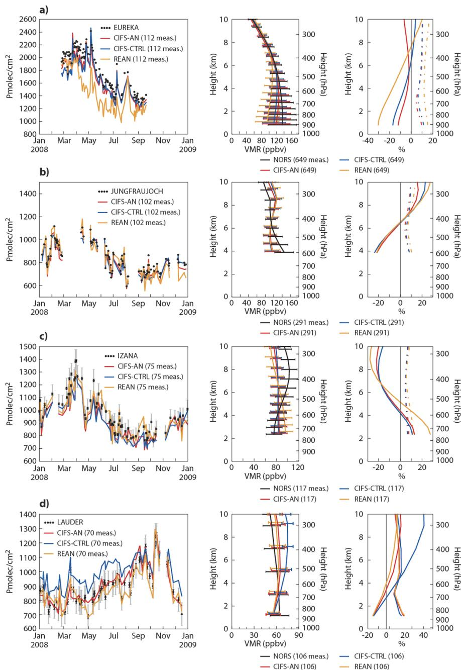
**Figure 6.** Time series of daily mean tropospheric CO columns (surface to 10 km) in  $10^{15}$  molecules  $\text{cm}^{-2}$  (left), annual mean CO volume mixing ratio profiles in ppbv (middle) and annual mean bias (model minus observation) profiles in % (right, with dashed lines for spread) for the year 2008 for four NDACC stations: (a) Eureka, (b) Jungfraujoch, (c) Izaña and (d) Lauder. CIFS-AN is shown in red, CIFS-CTRL in blue and REAN in orange.
