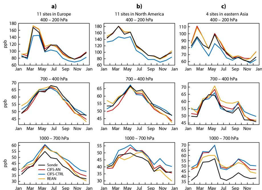
**Figure 14.** Time series of monthly mean tropospheric O<sub>3</sub> in ppb over (a) Europe (11 stations), (b) North America (11 stations) and (c) eastern Asia (4 stations) averaged in the pressure bands 1000–700 hPa (bottom), 700–400 hPa (middle) and 400–200 hPa (top) from ozonesondes (black), CIFS-AN (red), CIFS-CTRL (blue) and REAN (orange) in 2008.
