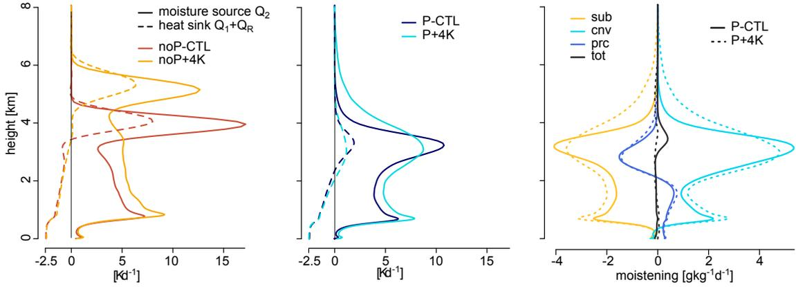
**Figure 2.7.:** Profiles of the heat sink ( $Q_1 + Q_R$ , dashed) and moisture source ( $Q_2$ ) for the CTL and +4K climate states of the noP cases (left, averages of day 7 are shown) and the P cases (middle). (right) Individual moistening tendencies of the P-CTL and P+4K simulations.
