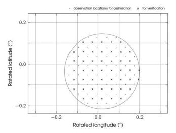
Fig. 5. Locations of thinned precipitation observations created for assimilation from data of the X-band radar at MOD site (Lengfeld et al., 2014) on a  $5000 \,\mathrm{m} \times 5000 \,\mathrm{m}$  grid (dots) and locations for verification on a  $5000 \,\mathrm{m} \times 5000 \,\mathrm{m}$  grid shifted by  $2500 \,\mathrm{m}$  north and east (crosses).
