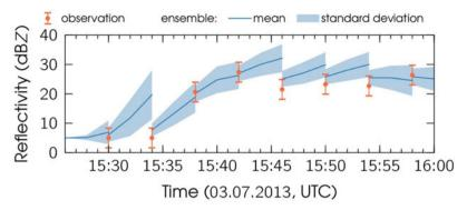
Fig. 7. Reflectivity ensemble mean evolution (dark blue line) and uncertainty range (light blue envelope,  $\pm$  one ensemble standard deviation) throughout the data assimilation cycle at observation grid point  $0.041^{\circ}$ E,  $-0.053^{\circ}$ N (indicated by a cross in Fig. 8) and observations (orange whiskers,  $\pm$  observation error standard deviation).
