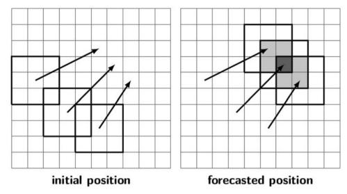
Fig. 3. Schematic representation of the forecasting step for three pixels, exemplary.  $3 \times 3$  windows of pixels (initial position left) are shifted according to the local motion vectors calculated for the middle pixel. If these pixel windows overlap in the forecast (new position right), pixel values (precipitation intensity or motion velocity) are averaged to get the forecasted field. In this example, light grey pixels are averages over two values, dark grey over three values.
