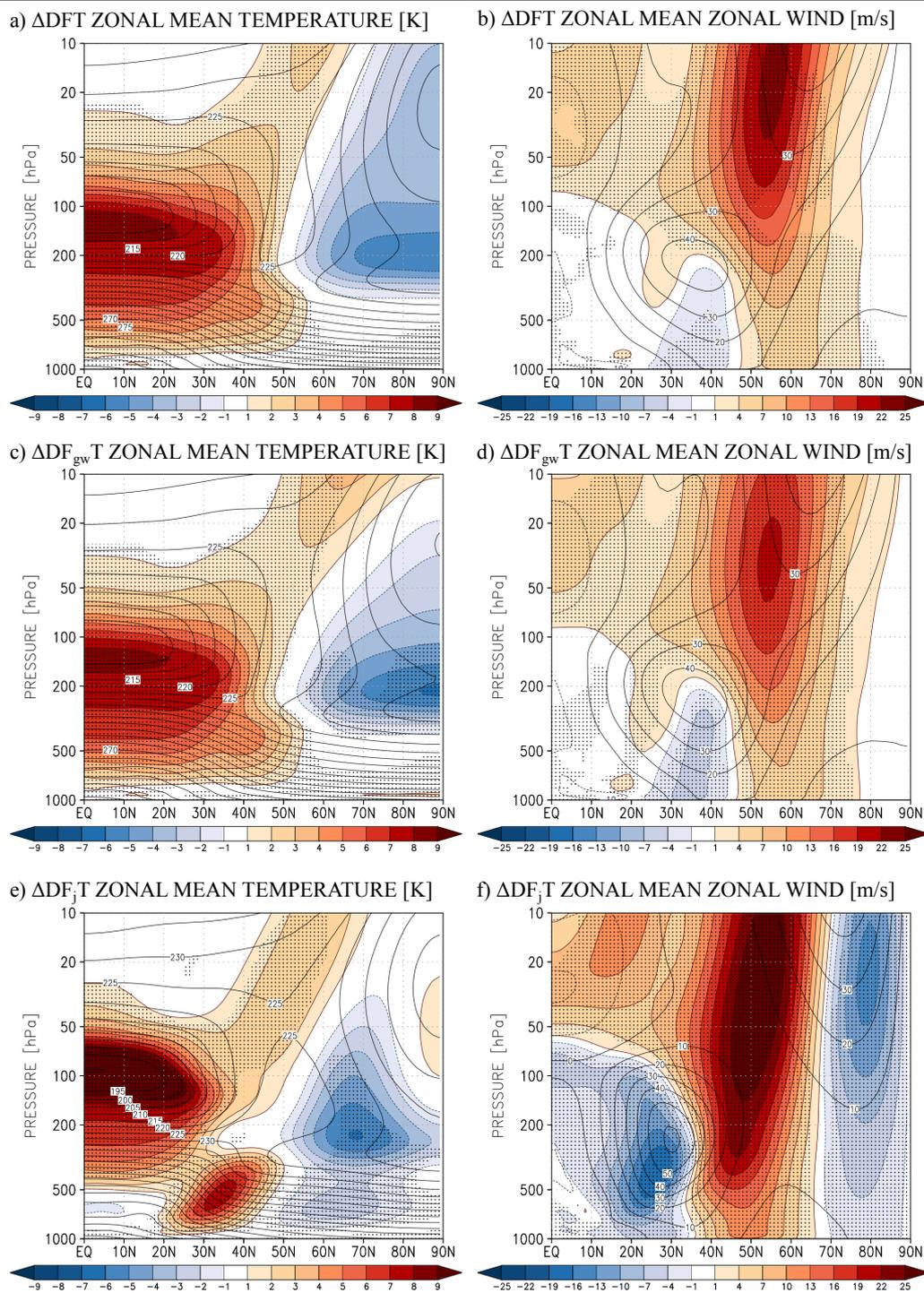
**Figure 3.1.**  $\Delta DFT$ ,  $\Delta DF_{gw}$  and  $\Delta DF_j$  steady state temperature [K] and zonal wind [m/s] change shown in color shading. Stippling mark areas where the change is significant using the 95<sup>th</sup> percentile threshold. Contour lines show the respective control experiment's steady state.
