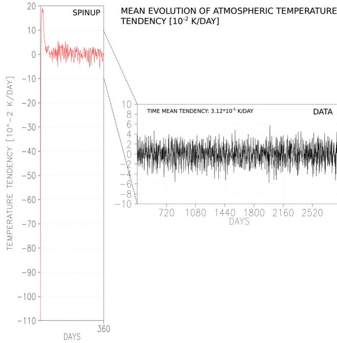
**Figure 2.6.** Domain mean temperature tendency evolution of the ICON-DRY's DF control experiment. The red line shows the spinup phase and the black line the data
