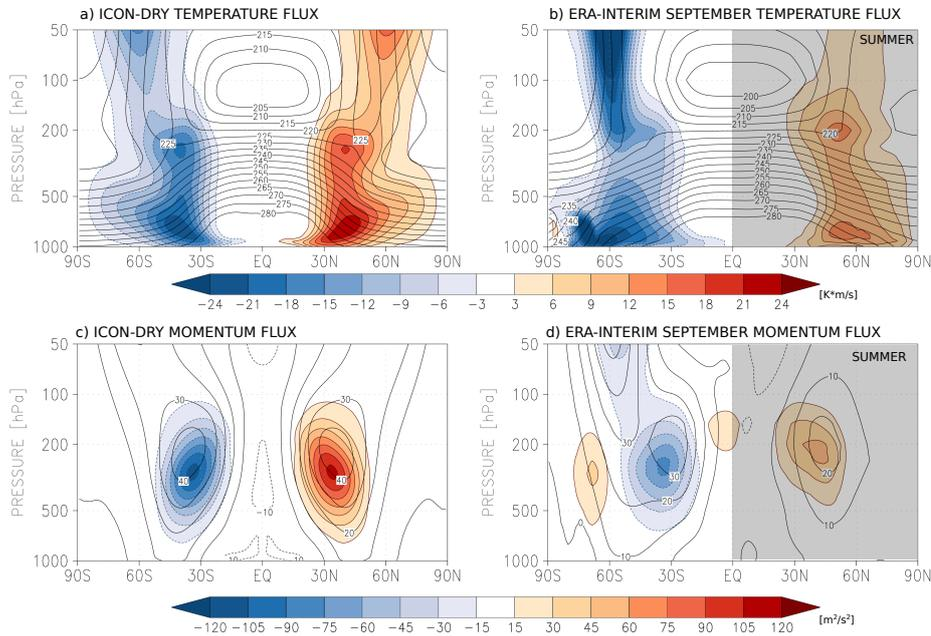
**Figure 2.10.** The upper row shows the time mean of the temperature flux together with the time mean of the temperature. The bottom row shows the time mean of the momentum flux together with the time mean zonal mean wind for a) and c) the DF control experiment and for b) and c) September ERA-Interim reanalysis. The Northern hemisphere is masked with a gray shading since the DC control experiment is more comparable to the southern hemisphere in terms of orography.
