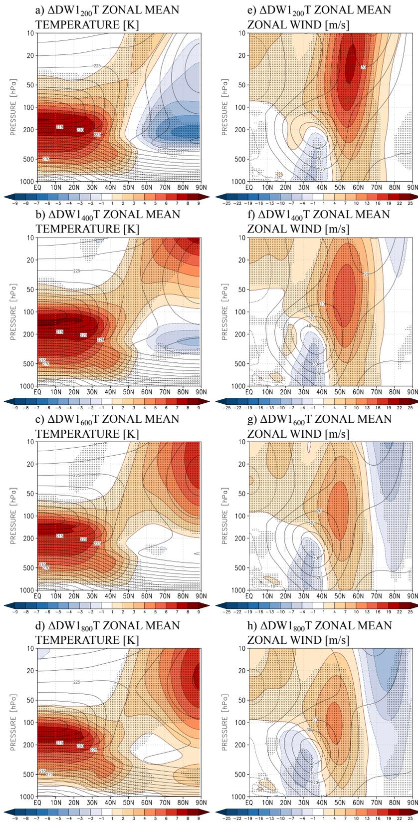
**Figure 4.2.**  $\Delta DW_{1_x T}$  steady state zonal mean temperature and zonal mean zonal wind response to tropical amplification. Countour lines show the control experiment's steady state.
