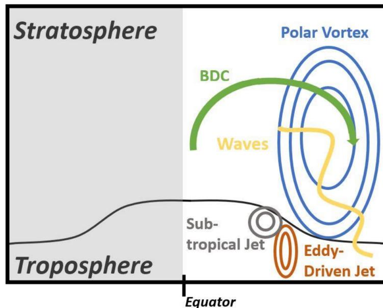
**Figure 1.1.** Sketch of the key elements of the tropospheric and stratospheric circulation. Depicted are the polar vortex, the subtropical jet, the eddy-driven jet, the Brewer-Dobson circulation (BDC) and the upward propagation of waves. The black line separating the stratosphere and the troposphere represents the tropopause region .
