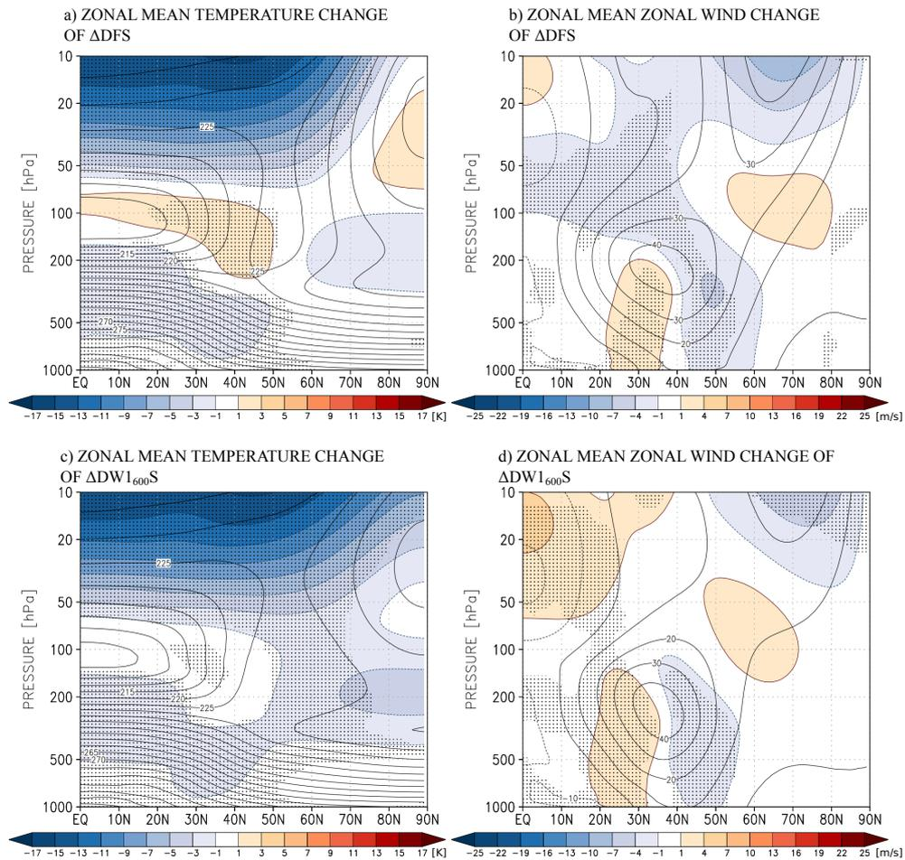
**Figure 3.15.**  $\Delta$ DFS and  $\Delta$ DW<sub>1600S</sub> steady state temperature and zonal wind change shown in color shading. Stippling mark areas where the change is significant using the 95<sup>th</sup> percentile threshold. The method used to calculate the statistical significance is explained in section 2.3.6. Contour lines show the control experiment's steady state.
