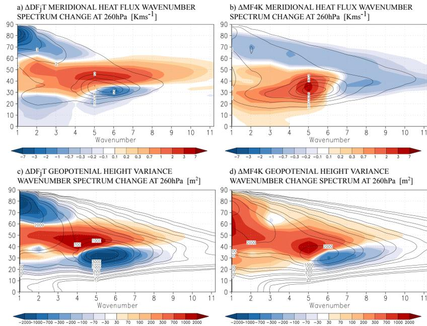
**Figure 3.6.**  $\Delta D_{jT}$  and  $\Delta MF4K$  mean heat flux (top row) wavenumber spectrum change and mean geopotential height variance (bottom row) wavenumber spectrum change at 260hPa shown in color shading. Contour lines show the respective control experiment's steady state.
