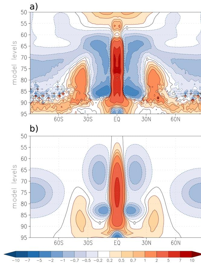
**Figure 2.4.** Sum of the heating rates due to evaporative cooling and diabatic warming, the water vapour related long wave radiation, the vertical diffusion difference and tropospheric short wave radiation in K/day (a). The tuned thermal forcing is shown in K/day in (b).
