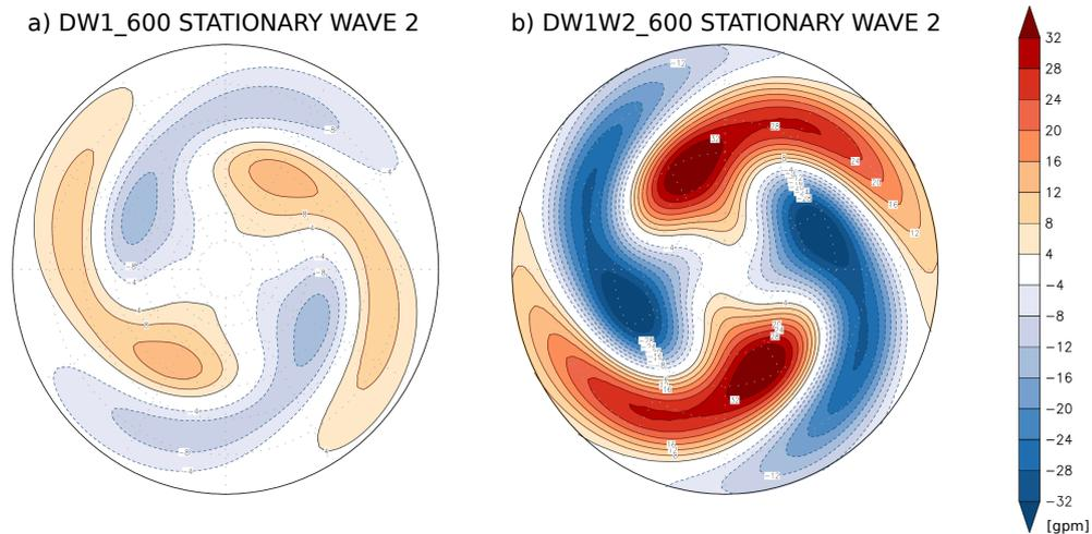
**Figure 2.9.** Polar stereographic plot of the filtered stationary wavenumber 2 at 500hPa for a) the DW1<sub>600</sub> control experiments and b) the DW1W2<sub>600</sub> control experiments.
