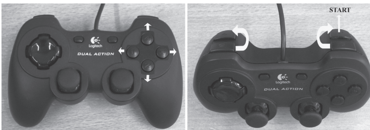
Figure 2. The Game Controller with four spatial buttons to move around the board (indicated in the front view) and with rotation buttons located on top of the controller (left/right, indicated in the top view). There was one start button on top of the controller below the right rotation button
