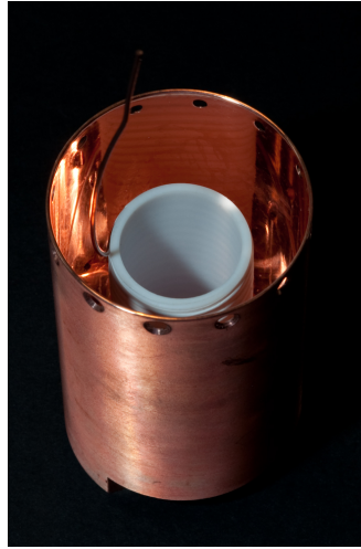
(b) Helical cyclotron coil in open housing. The coil is made from high-purity copper wire wound on a hollow teflon cylinder. The housing is made from OFHC copper. It is polished on the inside.
