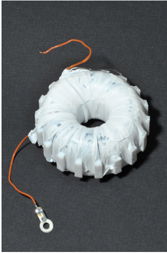
(a) Axial toroidal coil. The coil is made from 75 \mu\text{m} thick NbTi wire wound on a teflon torus. The torus is wrapped with teflon tape. The two copper wires soldered to the ends of the coil can be seen.
