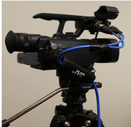
FIGURE 2. The JVC GY on a Velbon DV-6000 tripod with Velbon PH-358 panhead. Note the audio attachment/handle allows for the dual XLR inputs.
