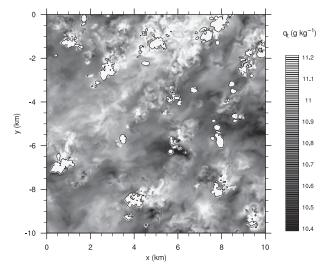
FIG. 17. Total water mixing ratio (grayscale contours) for case SMC-C-20-X on a horizontal plane at z = 1500 m, about the middle of the cloud layer. Only a quarter of the computational domain is shown. Black contours denote the saturation mixing ratio. Small-amplitude dispersive oscillations are discernible downwind (northeast) of the clouds [e.g., at (6, -4) and (9, -5) km]. The maximum and minimum of  $q_t$  on the entire plane are, 15.9 and 9.7 g kg<sup>-1</sup>.
