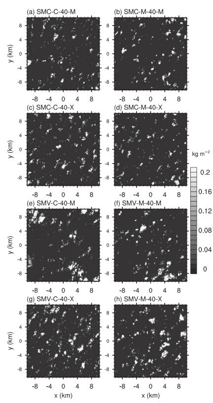
FIG. 2. Cloud LWP at the end of the simulation, t = 24 h. The panels of the left column correspond to LES with the nondissipative advection and show consistently higher cloud cover than those with the monotone scheme.
