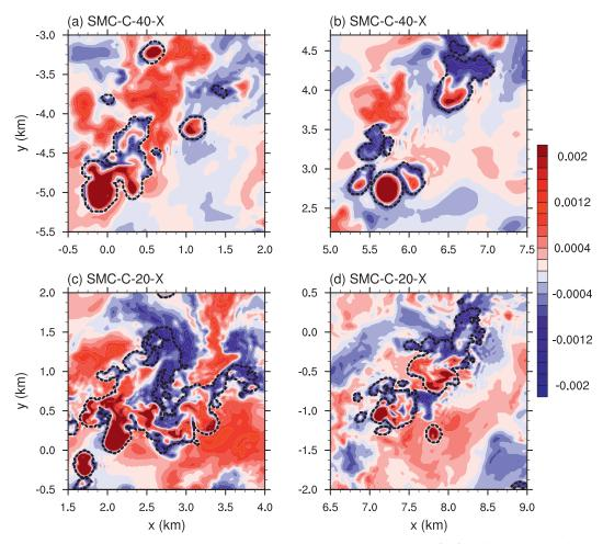
FIG. 16. Buoyancy at z = 1500 m for nonprecipitating cumulus convection cases at (top) medium resolution,  $\Delta x = 40$  m, and (bottom) high resolution,  $\Delta x = 20$  m. Black dotted contour corresponds to the saturation surface. Each panel shows a 2.5 × 2.5 km<sup>2</sup> subsection of the computational domain at t = 24 h. Note the thin negative buoyancy (dark blue contour) surface surrounding the clouds.
