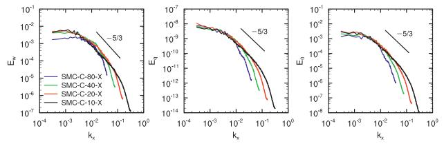
FIG. 12. One-dimensional power spectra along the zonal direction of vertical velocity, total water, and liquid water potential temperature at z = 1500 m.
