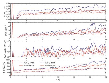
FIG. 1. Time evolution of cloud cover, LWP, surface precipitation rate, and vertically integrated TKE for runs with microphysics and  $\Delta x = 40$  m, for nondissipative advection (blue) and the dissipative monotone scheme (red), for SGS model implementation SMV (solid) and implementation SMC (dashed).
