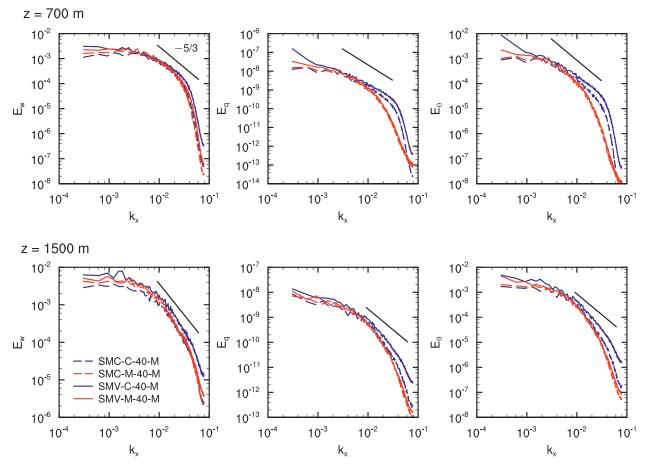
FIG. 5. One-dimensional power spectra along the zonal direction of (from left to right) vertical velocity, total water, and liquid water potential temperature for all runs with microphysics and  $\Delta x = 40$  m at the end of the simulation, t = 24 h, for (top) cloud base, z = 700 m, and (bottom) about the middle of the cloud layer, z = 1500 m.
