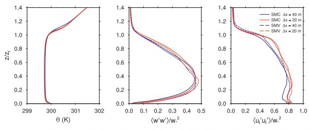
FIG. 14. Mean profiles for dry convective boundary layer runs with the two subgrid model implementations at two resolutions, 20 and 40 m. From left to right: potential temperature, vertical velocity variance, and resolved-scale TKE. The top of the computational domain is at  $z/z_i = 2.5$ .
