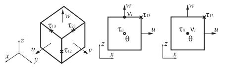
FIG. A1. (left) Variable arrangement on the computational grid. Scalar variables are denoted by  $\theta$  and the eddy diffusivity by  $\nu_t$ . (middle) Model SMV configuration; (right) model SMC.
