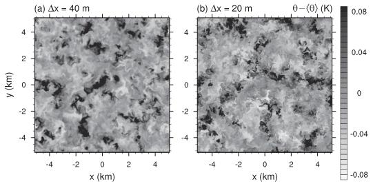
FIG. 15. Instantaneous potential temperature perturbation  $(\theta - \langle \theta \rangle)$  at half height of a dry convective boundary layer LES at two resolutions.
