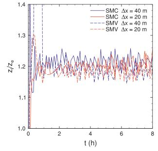
FIG. 13. Growth rate of a dry convective boundary layer computed with the two subgrid model implementations at two resolutions each.
