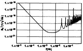
Figure 3. LISA estimated strain noise spectrum for an optimally oriented and polarized gravitational wave. The pattern of narrow insensitive bands at high frequency comes from the finite light travel time and washes out nearly completely for any source direction because of the antenna rotation when averaged over a year.
