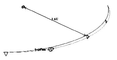
Figure 1. LISA orbits. The three spacecraft follow independent heliocentric orbits with parameters adjusted such that the distances among the spacecraft are kept constants to within  $\approx 1\%$  at  $5 \times 10^6$  km. The rotating triangle represents the laser beams joining the spacecraft located at the vertices. The drawing is approximately to scale. The Earth (not represented) leads the formation by 20°.
