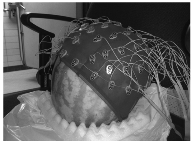
Fig. 2. To check for artifacts in the set-up, the experiment was also carried out with a watermelon phantom.
