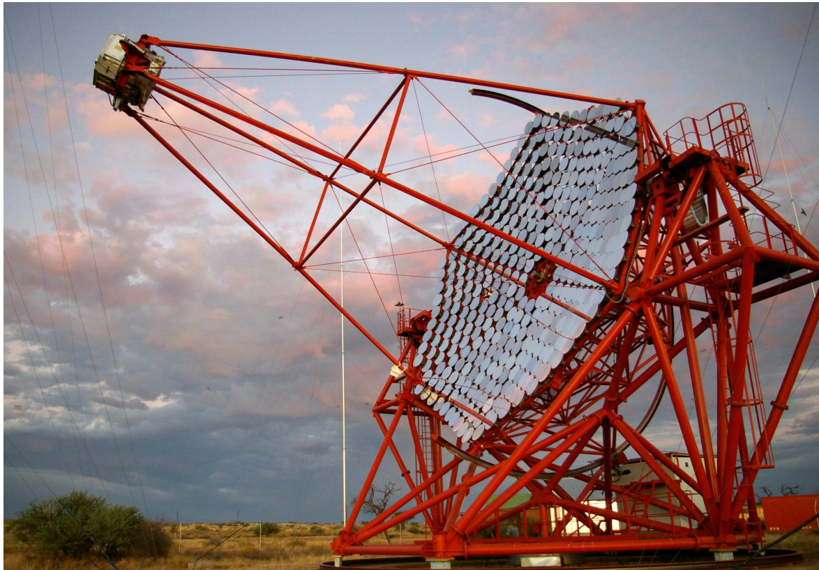
Figure 1.3: One of the four H.E.S.S. imaging atmospheric Cherenkov telescopes (IACTs) used to detect VHE \gamma -rays.
