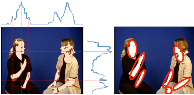
Figure 1: Left – a video frame with skin color pixels marked and histograms of those in two dimensions, X and Y. Right – example of ellipses approximating the skin areas in given image.
