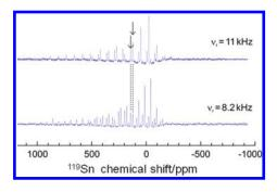
**Figure 3.** <sup>119</sup>Sn solid-state NMR cross-polarization spectra of bis-(stannylene) **2.** The spectra were recorded at 8.2 and 11 kHz MAS on a 9.4 T spectrometer. Isotropic chemical shifts are indicated by arrows.
