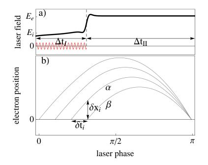
FIG. 1: Schematic of the recollision scenario: a) A half cycle of the tailored laser field (black). The red line is the assisting x-ray pulse. b) Different classical trajectories in the field of (a) which start into the continuum at different times but revisit the ionic core at the same time.
