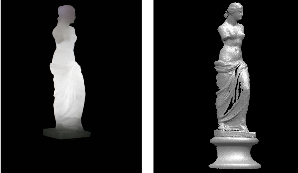
Figure 6.1: By combining phase-shifting and polarization our method faithfully captures the 3D geometry of very translucent objects such as this alabaster Venus figurine (height \approx 19\text{cm} ).
