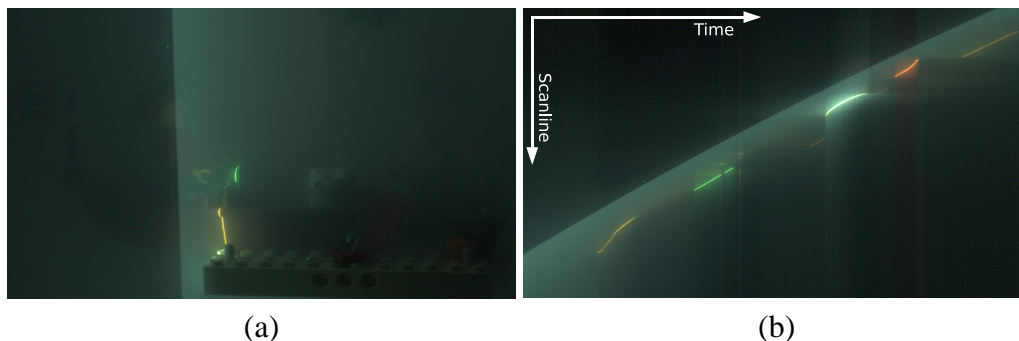
Figure 5.5: (a) A single vertical line projected into the island scene of Figure 5.1. (b) A horizontal slice of the recorded reflectance field. The opaque surfaces are clearly visible as well as the haze due to the scattering fluid.
