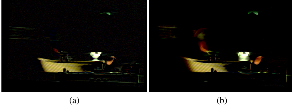
Figure 5.9: (a) A bright illumination plane in front of the considered confocal plane will darken the image region if a symmetric descattering kernel is applied. (b) The one-sided kernel neglects those planes, rendering a slightly brighter image of the internal structures and resulting in more recovered detail.
