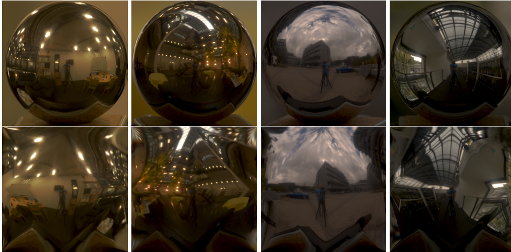
Figure 3.6: Example environment maps. The top row shows the images as they were acquired. The mirroring sphere shows the surrounding environment for the full hemisphere directed at the camera. The bottom row shows the environment maps in the hemi-octahedral representation where the sphere is unrolled onto a flat surface with simple boundary extension and without distortion.
