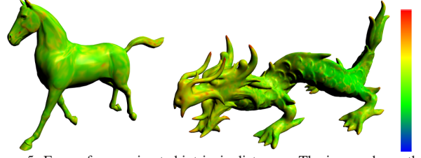
Figure 5: Error of approximated intrinsic distances. The image shows the maximum error over all geodesics between each point and all other points of the point cloud. Horse : 8431 original points, 1355 sample points - max error is 5% of the bounding box size. dragon : 20002 original points, 1598 sample-points - max error is 10%.
