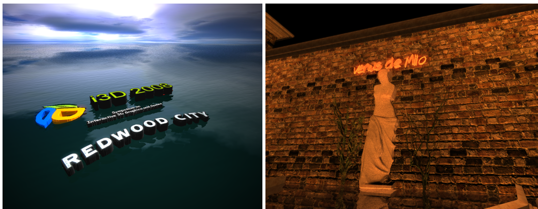
Figure 1: Left: Scene rendered with around 40FPS at 1500 \times 1200 screen resolution. The resolution of the height map is 1024^2 . The height field is rendered twice since water is reflecting the environment. Right: A screenshot from the Venus scene showing a highly complex height map applied on a planar surface, height map resolution is 4096^2 rendered with 25 FPS at 1200 \times 900 screen resolution.
