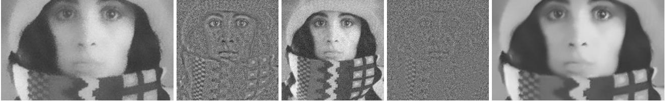
Figure 2: Center: "Trui" image corrupted by noise. Left: smoothed by bilateral filtering; the difference between the original noisy and smoothed images contains important image structures. Right: smoothed by NL-means filter of Buades, Coll, and Morel; the difference between the noisy and NL-smoothed images contains much less features of the original image. Thus the NL-means filter does a much better denoising job than the bilateral filter.
