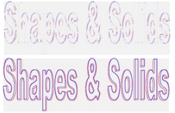
Figure 2: Crest lines detected on 3D text. Top: polynomial fit without preliminary estimation of mesh normals is used. Bottom: the enhanced adjacent-normal cubic approximation method is employed for estimating surface curvatures and their derivatives. In both the cases preliminary smoothing \mathbf{p} \rightarrow \mathbf{p}' was applied.
