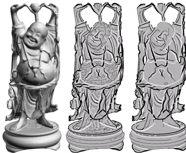
Figure 3: Filtering ridges (black) and valleys (white) according to their strength controlled by parameter T . Middle: T = 0 . Right: T = 2 .
