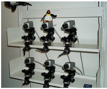
Figure 1. The Lumi-Shelf setup records three synchronized stereo-image pairs. Distributed processing of the video data enables interactive frame rendering rates.
