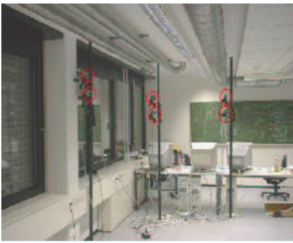
Figure 8. For combining visual hull reconstruction with depth map estimation, six cameras are grouped in pairs of two. The camera pairs are distributed along a 90^\circ -wide arc about the scene. Silhouette extraction is performed on the client PCs. The outlines are sent to the server to compute the polyhedral visual hull that is sent back to the clients. There, the visual hull is used to guide depth estimation for the object pixels. Object pixel color and depth is finally sent back to the server for rendering.
