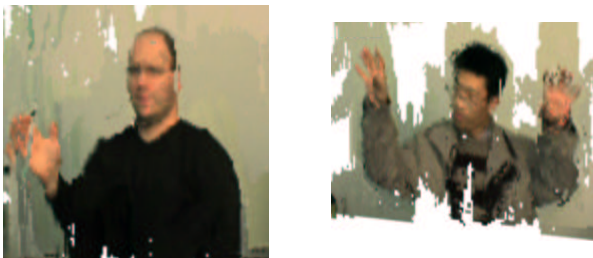
Figure 2. 3D-warped intermediate views using depth maps estimated on-line: Missing depth estimates lead to holes, while erroneous pixel depth values introduce isolated pixels.
