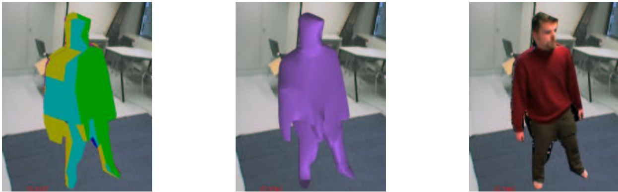
Figure 11. The visual hull is represented by the polyhedron resulting when intersecting the back-projected silhouette polygon cones. The surface can be arbitrarily shaded, or the video images can be applied as view-dependent textures by projective texture mapping in conjunction with shadow mapping to avoid through-projection artifacts.
