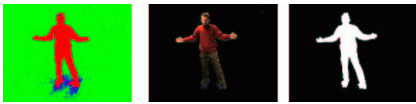
Figure 5. From pre-acquired background images, the dynamic foreground object is segmented exploiting statistical differences in pixel color.
