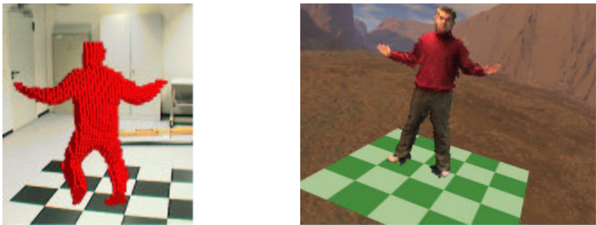
Figure 12. A volumetric model of the dynamic visual hull is reconstructed on-line. The voxel model is view-dependently textured by rendering each voxel as a billboard facet.
