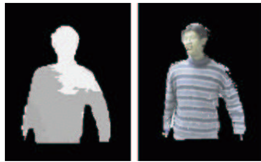
Figure 10. A dense depth map is obtained for the segmented foreground object at 4 frames per second by using the object's visual hull to initialize and restrict depth estimation.
