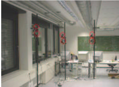
Fig. 1. Acquisition setup: 3 camera pairs are arranged along an arc.
