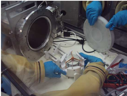
Figure A.31: The BEGe detector in a clean-bench, being prepared for transfer in the transportation lock (on the left).
