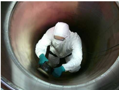
Figure A.3: Grinding of the cryostat inner wall at MPIK Heidelberg (June 2009).
