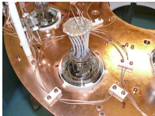
Figure A.12: Top view of a PMT and its voltage divider. The cables are guided on the copper plate by Teflon® clamps.
