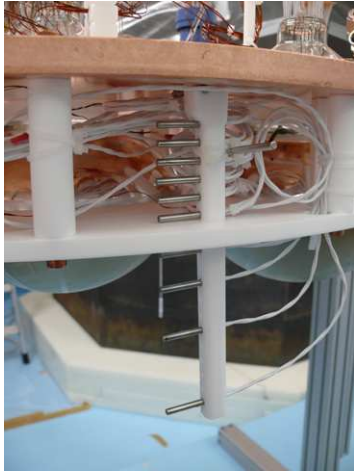
Figure A.13: Twelve PT1000 temperature sensors are attached at the side to monitor the LAr filling level.
