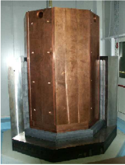
Figure 2.2: The LArGe passive shield during construction. All four layers depicted in figure 2.3 are visible.
