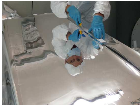
Figure A.6: Cutting of VM2000 mirror foil during the LArGe assembly in GDL (August 2009).
