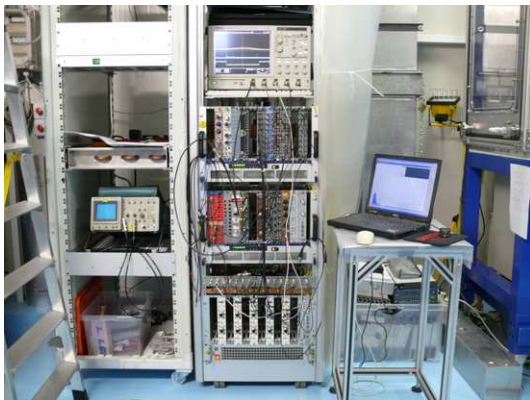
Figure A.33: The electronics of the DAQ system for PMT measurements.
