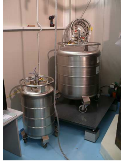
Figure A.26: The 400 l nitrogen dewar for the active cooling system on a scale, and the 120 l substitute dewar (both still unconnected).
