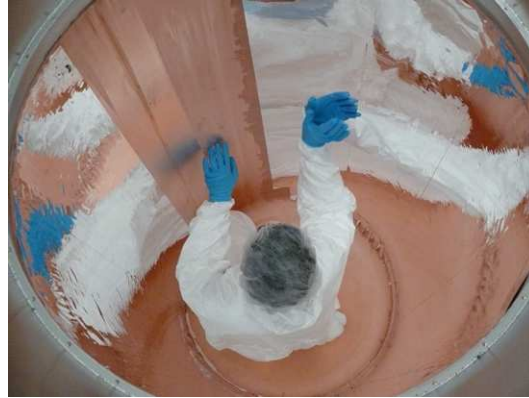
Figure A.8: ... and the VM2000 pieces are attached. Care must be taken to avoid air bubbles, which can contaminate the argon.
