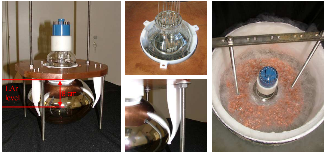
Figure 2.6: Left: PMT support mockup. The range of the LAr filling level between copper plate and PMT equator is indicated. Center top: ductile Teflon® collar. Center bottom: Teflon bracket. Right: mockup submersed in LN 2 .
