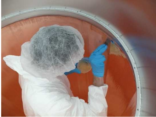
Figure A.7: Lining of the cryostat with mirror foil. A thin layer of two-component epoxy resin (Araldit) is applied...
