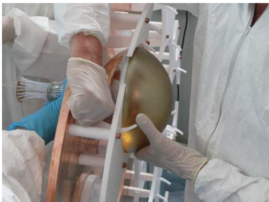
Figure A.11: Insertion of a PMT. Each PMT is hold by three thin Teflon® brackets, which grab the edge of the photocathode.
