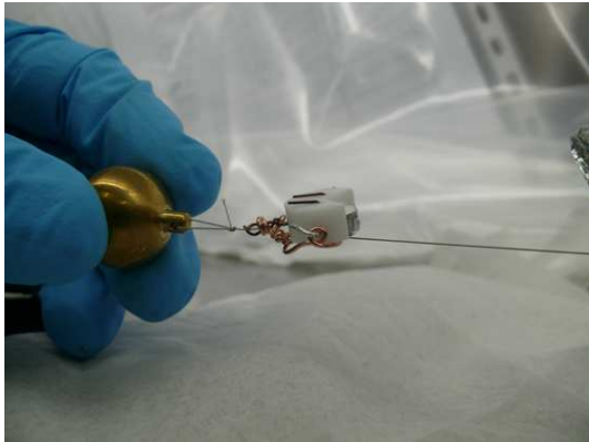
Figure A.27: A ^{148}\text{Gd} alpha source on its Teflon holder, and a brass weight.
