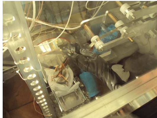
Figure A.32: A view into the main lock, while preparing the detector string of BEGe for submersion into the cryostat.
