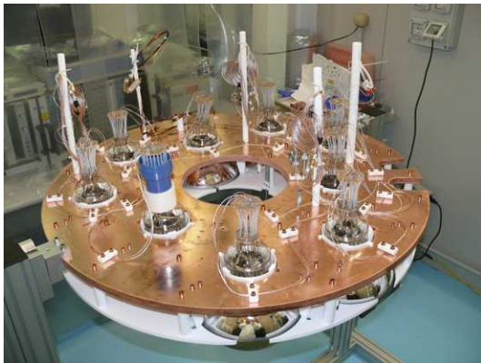
Figure A.15: The PMT support structure ready for insertion into the cryostat.
