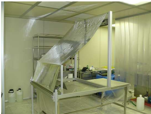
Figure A.5: The first wavelength-shifter coating-machine with a freshly laminated piece of mirror foil (March 2008).
