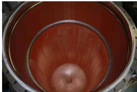
Figure A.4: A view into the cryostat after etching (July 2009).
