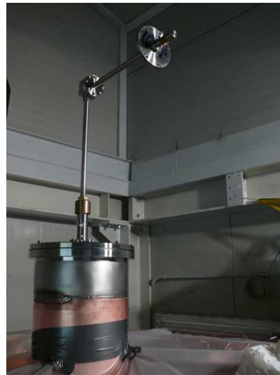
Figure A.28: The alpha-source manipulator mounted on the 'access cylinder' of the cryostat.
