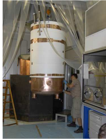
Figure A.2: Insertion of the cryostat into the shield. The cryostat is wrapped in Styropor® for better insulation.
