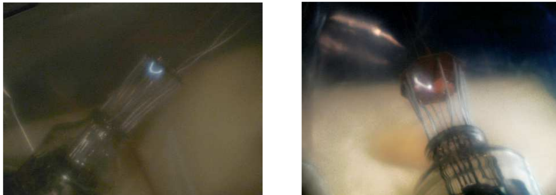
Figure 2.14: Pictures of spark discharges on the PCB in argon gas atmosphere. Each picture is an overlay of two images from the same camera angle: one taken in darkness while sparking occurs; the other one at light, to locate the spark position on the PCB.
