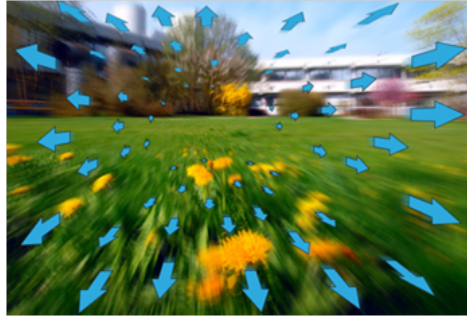
Figure 1.1: Illustration of Optic-Flow. Self-motion causes a permanent shift of the images on the retina. The resulting pattern of local velocities (represented by the arrows) is called optic-flow. The image illustrates the optic-flow induced by a forward translation.
