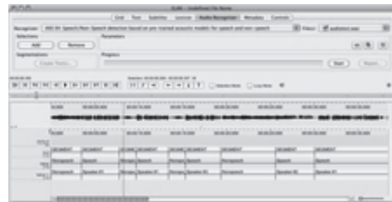
Figure 1: Three layers of annotation representing three steps of the automated analysis. First layer is the result of the uniform document segmentation, second layer is the division into speech/no-speech parts, third layer recognizes different speakers in the recording. All the steps have been performed automatically
