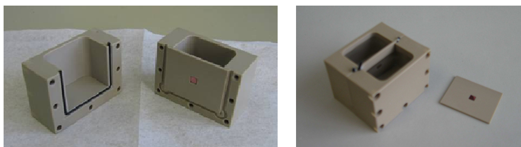
Figure 2.21 Photograph of PPC measurement cell made of organic polymer thermoplastic, polyether ether ketone (PEEK)
