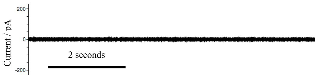
Figure 6.8 Leakage current measurement of a side-wall electrical passivated membrane chip at applied +100 mV DC
