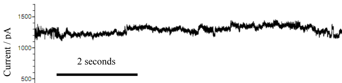
Figure 6.5 Leakage current of a membrane chip (without electrical passivation) against time at applied DC holding potential of +100 mV
