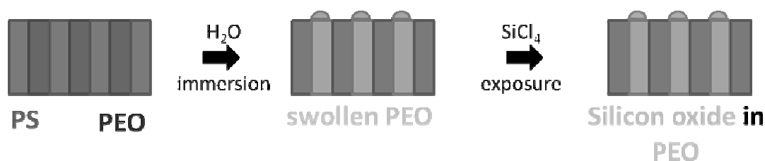
Figure 14: Using PEO- b -PS scaffolds to grow silicon oxide particles from the swollen PEO domain (adapted from literature 108 )
