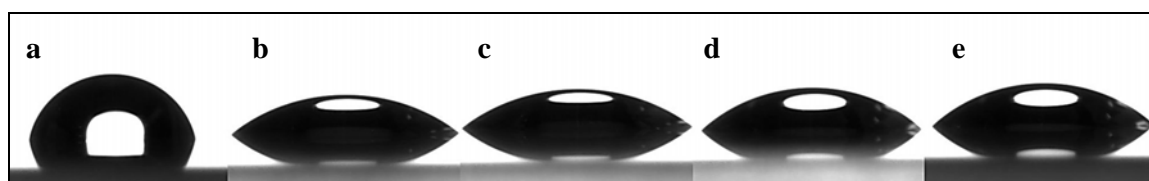
Figure 3.2 CCD images of (a) bare gold, (b) 20min, (c) 45min, (d) 120min, (e) overnight incubation period of 0.01mg/ml P19
