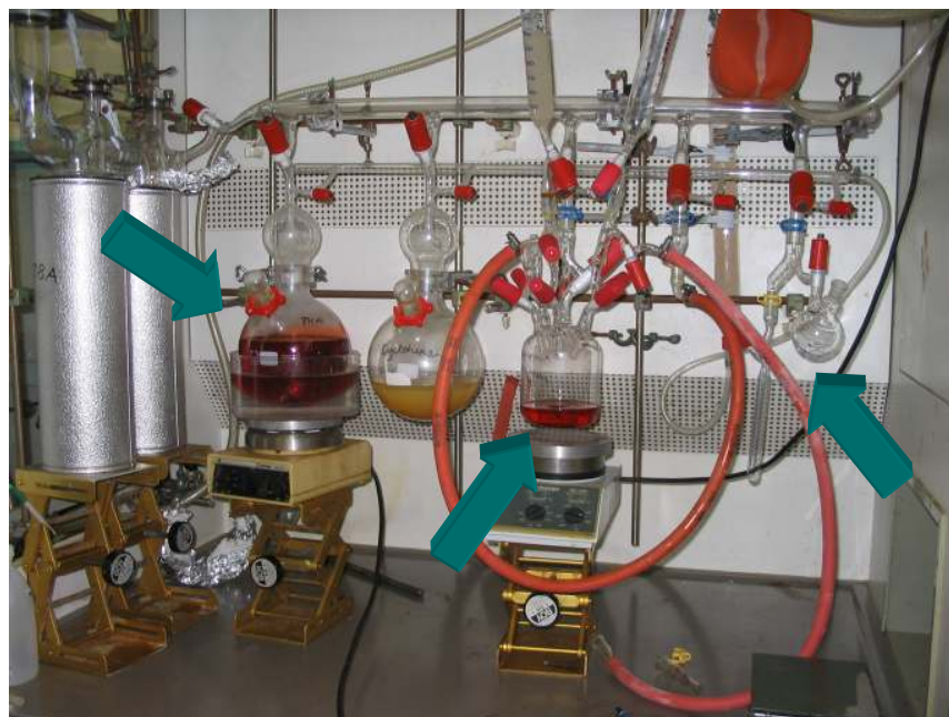
Fig. 12.1.4.3.: High vacuum anionic polymerization line with solvent reservoirs (left arrow, reactor (middle arrow) and vacuum distillation setup (right arrow).
