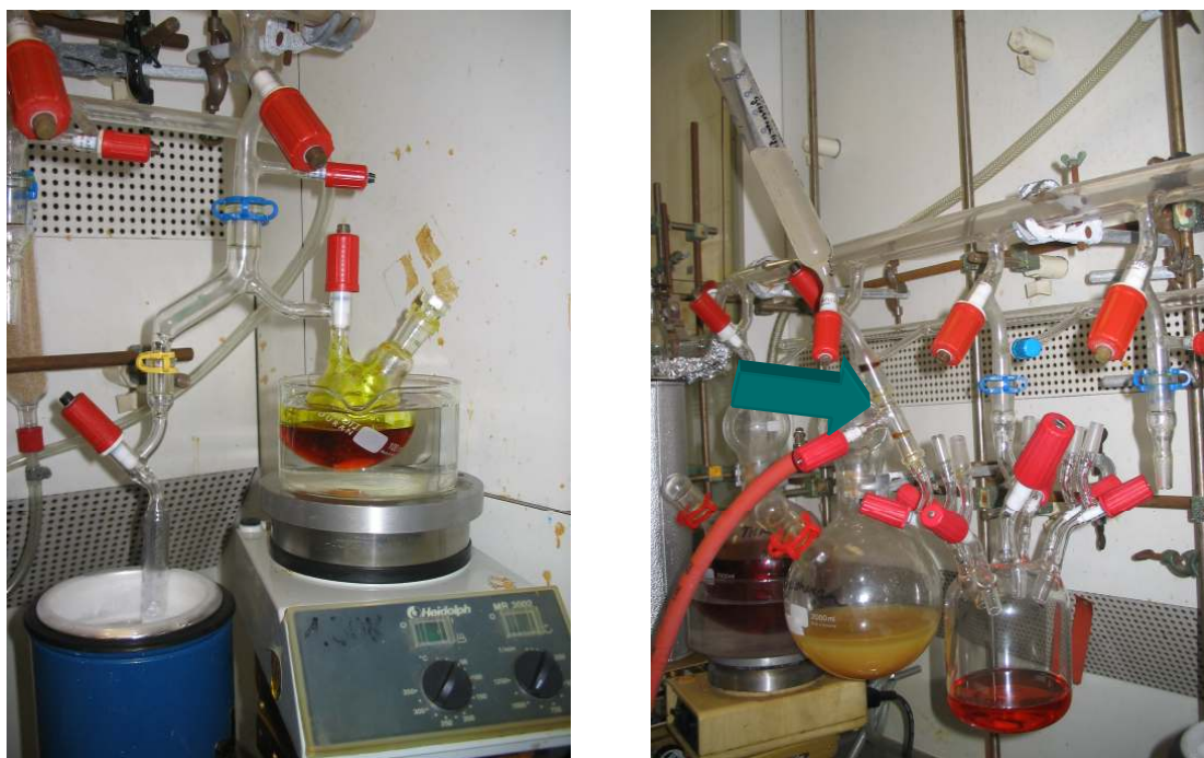
Fig. 12.1.4.4.: Monomer distillation (left), reagent addition to anionic polymerization reactor via Schlenk technique (right)
