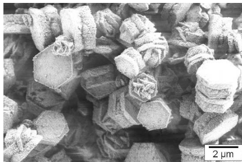
Figure 3.7. ZnO precipitated in the presence of 1 \text{ g L}^{-1} of the latex LT6 (cf. Table 2.4), which was prepared without addition of \text{K}_2\text{S}_2\text{O}_8 in advanced states of the polymerization.
