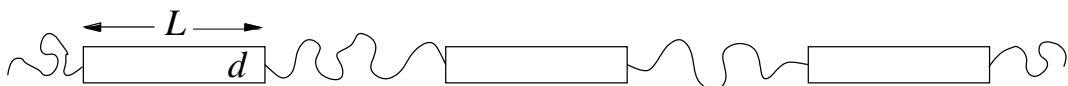
Figure 1.3: This figure shows a rod-coil multiblock copolymer with rods of length L and diameter d . The stiff rods are connected by flexible chain parts.
