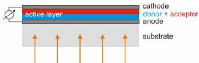
Figure 1-16: Schematic presentation of the setup of a heterojunction photovoltaic device.
