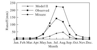
Figure 2. Simulated monthly average runoff (mm) by using Model II, the mixture (mm) of meltwater simulated by Model I and runoff in the unglacierized area simulated by Model II during 1970 to 1997, and runoff observed (Archer, 2003) at Dainyor Station during 1966 to 1997 in Hunza River Basin.
