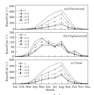
Figure 5. Monthly runoff (m<sup>3</sup> s<sup>-1</sup>) in the (a) glacierized, (b) unglacierized, and (c) total areas if air temperature increases by 0, 1, 3, 5, and 7 °C, respectively, above Lake Gojal in Hunza River Basin.
