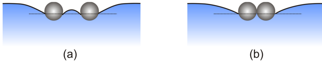
Figure 7: (a) Meniscus formation at the colloid, air and water interface. (b) The total meniscus decrease due to the formation of closely packed colloids.
