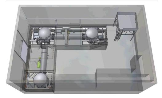
**Figure 1.** The vacuum system is set up in the downstairs area of the AEI prototype hall. The upstairs area is used for assembly of mechanical components before installation as well as for other optical experiments.
