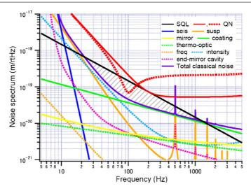
**Figure 3.** The design sensitivity of the AEI 10 m prototype interferometer. The black straight line is the SQL, the red solid curve is the sum of quantum noise, the blue solid line is the sum of all classical noise sources. The dashed area inbetween the sum of classical noise and the SQL is the QND regime that we hope to be able to explore by applying e.g. the back-action evasion technique (red dashed curve).
