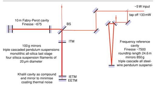
**Figure 2.** The basic optical layout for the first round of experiments in the AEI 10 m prototype facility. The frequency reference cavity and the main interferometer along with the most relevant design parameters are shown. Note that only 5 W input power will be used for the first experiments.
