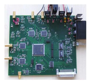
**Figure 3.** 4-channel prototype of LISA Phasemeter with extended signal processing and readout opportunities. EPP with output rate up to 1 MB/s. Digital input/output (DIO) with maximal rate of 2 GB/s.
