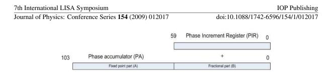
Figure 2. Phase reconstruction using phase accumulator.
