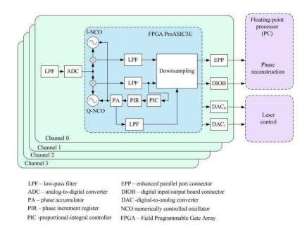
Figure 1. Block diagram of the phasemeter core design.
