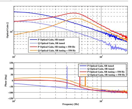
**Figure 5.** Measurement of the optical gains for tuned and detuned signal recycling for the two orthogonal quadratures P and Q. For the tuned case the demodulation phase was not optimized. Therefore the differential armlength signal is still clearly present in the optical gain of the Q-signal.
