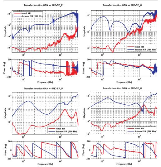
**Figure 6.** Measurements of the transfer functions from oscillator phase noise (OPN) and oscillator amplitude noise (OAN) to the error signal of the differential arm length servo. The red trace represents tuned signal recycling, while blue indicates a detuning of 510 Hz. The magnitudes of transfer functions are normalized by magnitudes of the optical gains from figure 5.
