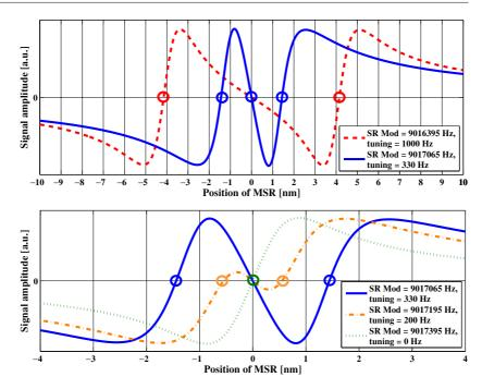
**Figure 3.** Signal recycling error signals derived from an RF modulation demodulation technique versus microscopic position of the signal recycling. The error point is plotted for various modulation frequencies corresponding to detunings of the signal recycling cavity between 1000 Hz and 0 Hz. By increasing the modulation frequency the structure gets more and more squeezed.
