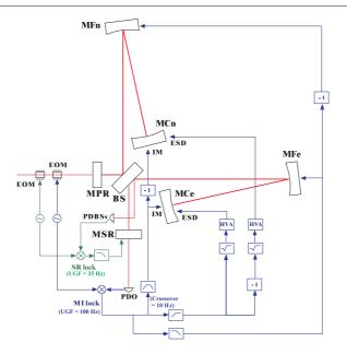
**Figure 2.** Simplified control scheme for two longitudinal degrees of freedom of GEO 600. Shown are the Michelson differential loop and the signal recycling loop in blue and green, respectively. The control signals used for lock acquisition are not shown in the diagram.
