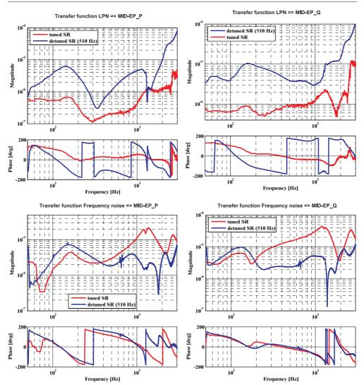
**Figure 7.** Measurements of the transfer functions from laser frequency noise and laser power noise to the error signal of the differential arm length servo. The red trace represents tuned signal recycling, while blue indicates a detuning of 510 Hz. The magnitudes of transfer functions are normalized by magnitudes of the optical gains from figure 5.
