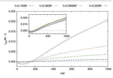
**Figure 1.** Error  $r_{AH}/M - 2$  in the areal radius of the apparent horizon as a function of time for evolutions of Schwarzschild initial data at four different resolutions. The main figure shows  $r_{AH}/M - 2$ , while the inset shows  $(0.1M/h)^4 \times (r_{AH}/M - 2)$ , demonstrating that the error shows fourth-order convergence to zero as the resolution is increased.
