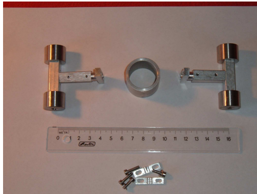
Figure 3.3.: Photo of the last pendulum stage. The hollow cylinder in the center hosted a standard 1 inch optical mirror. The two additional wings increased the overall moment of inertia, thereby reducing the resonance frequencies of the system.
